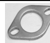
Part Number# FX04 Oval, 2-Bolt Flanges, 1.875 Center Hole, 3.250" Center Line, 0.500"x0.750" Slots Bolt Hole Size
