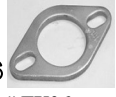
Part Number# FX06 Oval, 2-Bolt Flanges, 2.120 Center Hole, 3.500" Center Line, 0.500"x0.750" Slots Bolt Hole Size
